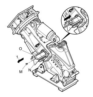
■ Disassemble the bolt cage (N).
