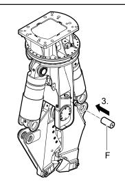
Place the hydraulic demolition cutter with the broad back of the cutter jaw (double) on the assembly rack so that the pin lies in the semi-shell of the assembly rack.
