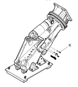
The bolt cage has two Allen screws.
