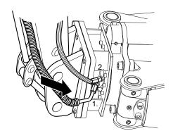
Connect both hoses for the function »Turn« at the boom, torsion-free.
