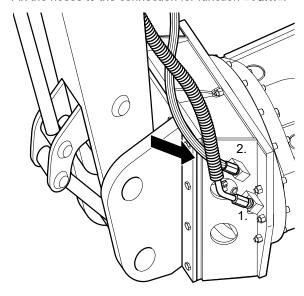
Connect both hoses for the function »Turn« at the boom, torsion-free.
