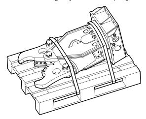
Move the fork of the forklift truck under the pallet so that the hydraulic attachment cannot tip over.
