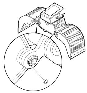
• Replace damaged castle nuts and splint pins.
